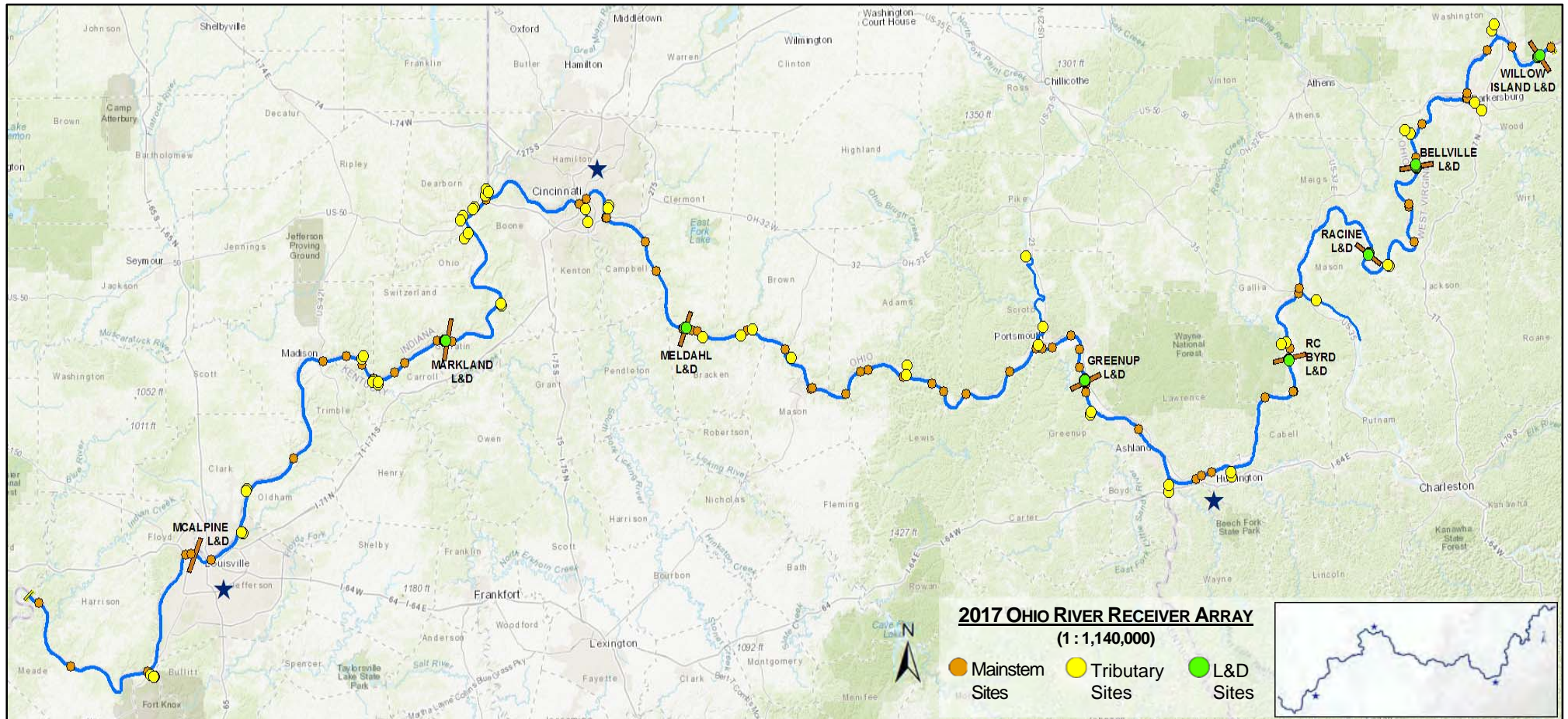
Figure 1. A map of the project’s entire 500-mile telemetry array with the eight separate Locks and Dam locations that are monitored for upstream/downstream transfers of tagged Asian Carp. The 2017 array included 158 receiver stations that were distributed across three distinct habitat types, which included the mainstem river, the tributaries, and the L&D’s.
