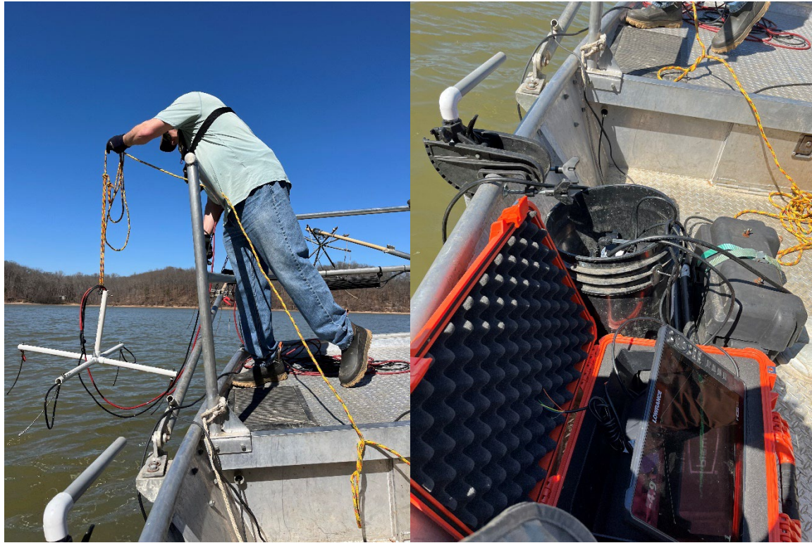
Figures 7 (left) and 8 (right). Example of Murray State University's dropper for deepwater electrofishing rig (Figure 7). The FFS system is used in conjunction with the dropper to ensure fish are targeted with the small field (Figure 8), so that the boat used turns on and off the electricity to more effectively obtain fish. The transducer is clamped to the gunwale of the boat and can freely rotate to help initially find structure to target fish on.
