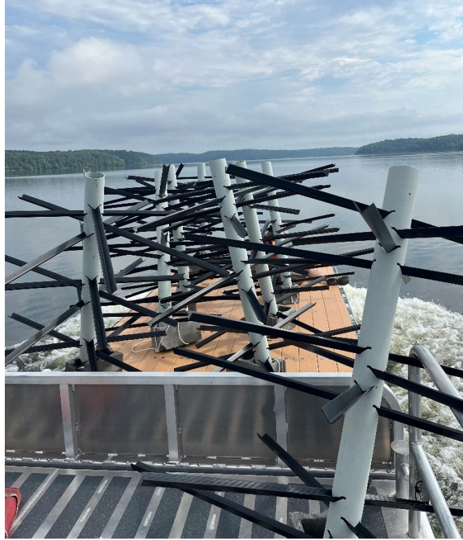
Figure 11. Photo of Mossback Trophy Tree XLs on dump barge being transported to drop site on Kentucky Lake. An example of a technical guidance project. This project only took one day to drop 75 structures between 5 sites.
