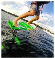
Hydrofoil - a vessel that consists of a board fitted with a mast extending below the board that is attached to a fuselage with a forward wing and a rear stabilizer.
