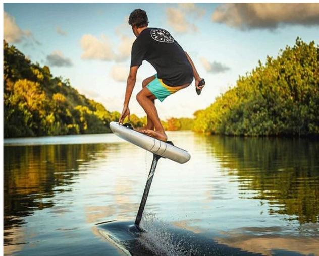
Mechanically Propelled Personal Hydrofoil (MPPH) – also known as an e-foil, is a vessel that consists of a board fitted with a mast extending below the board that is attached to a fuselage with a forward wing, rear stabilizer, and electric or internal combustion engine.
