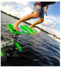
Hydrofoil - a vessel that consists of a board fitted with a mast extending below the board that is attached to a fuselage with a forward wing and a rear stabilizer.
