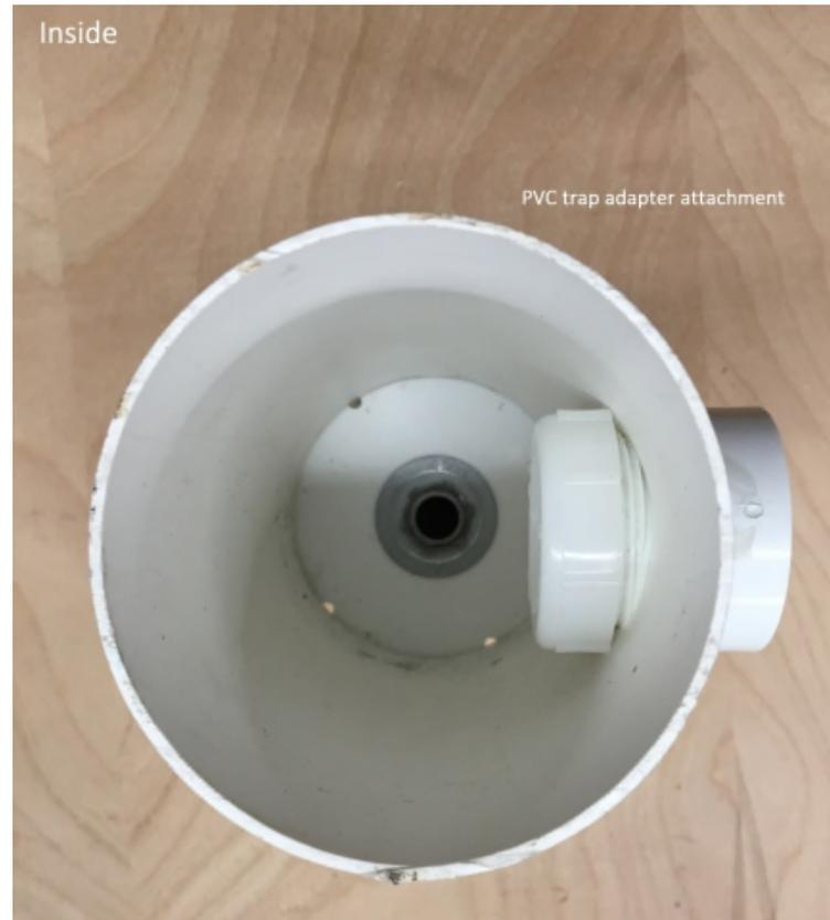
**Step 3: Conduit connector** – using a 13/16" drill bit, drill a hole in the center of one of the 4" PVC end caps, this will become the bottom of the box. Slide the conduit connector through the cap, with the threaded end inside the cap. Place the reducing washer over the connector on the inside of the cap. Then tighten down the supplied conduit connector washer using an adjustable wrench or ratchet and socket.
