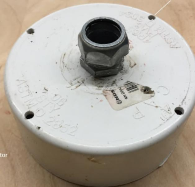
View of conduit connector attachment
