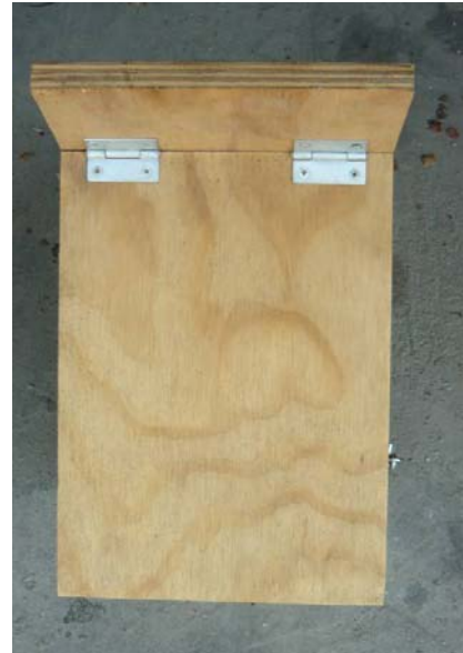
Figure 3. A view looking down at the roof of the box. Hinges are attached at the rear of the roof to allow access. The rear edge of the roof is cut at an angle to allow the roof to meet up flush with the back.
