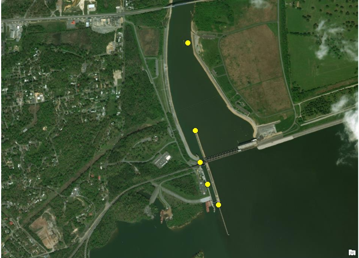
Figure 5. Yellow dots indicate location of passive VR2W receivers deployed around the Lake Barkley Dam and tailwaters.
