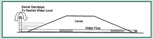
Figure 4. PVC pipe with 90-degree elbow and standpipe.
