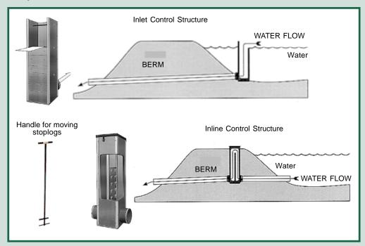
Figure 3. Prefabricated inlet and inline box type flashboard risers. Web site images courtesy of Agri Drain Corporation at www. ad-copr. com
